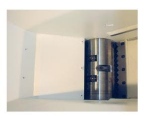
The rugged rotor bearings are a guarantee for smooth shredder running. The encapsulated bearing prevents material or other foreign bodies from penetrating the bearing housing.
